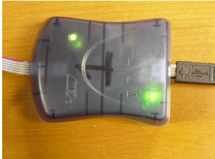
Figure 9 - AVRISP mkII Programmer Correctly Connected to Controller
