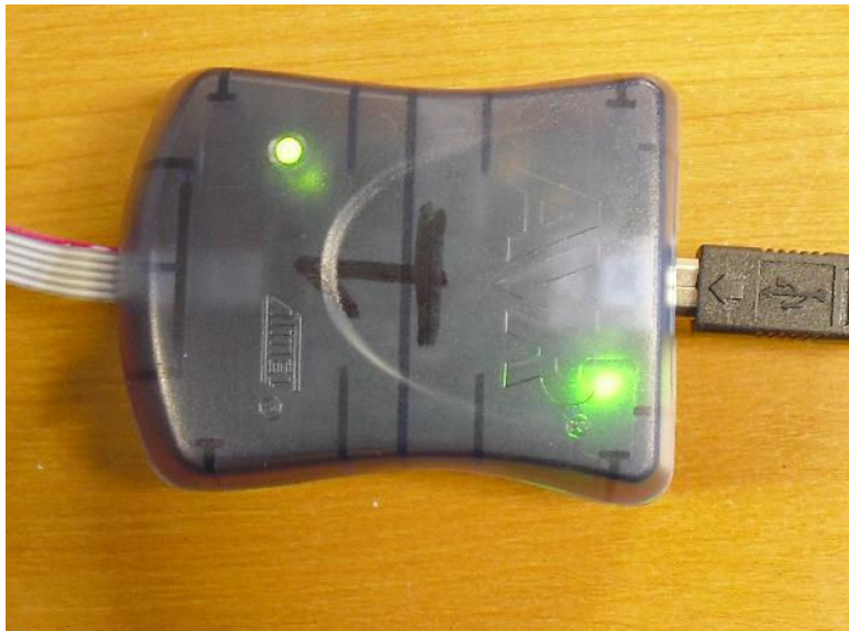
Figure 4 - Atmel's AVRISP mkII Programmer
