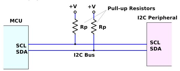
Again, this is part of the I2C specification, and not a "CEENBoT thing". The resistance value to use for the pullups is traditionally around ~1.5K ohms. However, before you immediately make the decision to use 1.5K ohms, just because I said so, you *really* should read the following introductory and insightful article regarding resistor pull-ups and the I2C bus: <u>http://www.dsscircuits.com/articles/effects-of-varying-i2c-pull-up-resistors.html</u>.
