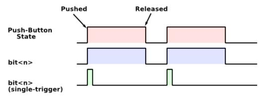
The *pink* graph is what the user is doing physically with the push-button. The *blue* shows how the bit logic values reflect what the user is doing physically (bits 2-4). The *green* shows how this same information is conveyed for the *edge-triggered* bits (bits 5-7).
