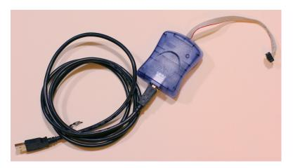
2) Hook up the ISP connector to the CEENBoT's '324 board as shown:
