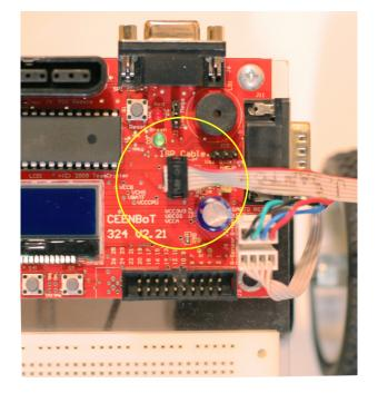
3) While we're here, right above where the ribbon cable connects is a small *header* with three pins as shown in the below figure, labeled **J2**:
