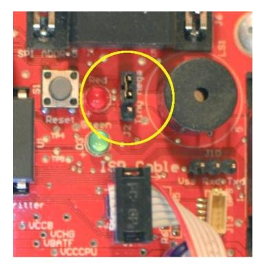
Although difficult to see in the above figure, one of the pins is fully *exposed*, while the remaining two are not. Next to this 3-pin header are the labels "**Tiny**" and "**Mega**". Your *mission* – should you choose to accept it – is to make sure that the two pins next to where it says "**Mega**" are the ones *covered* by the black "Jumper", while the lower pin, next to where it says "**Tiny**" remains exposed.
